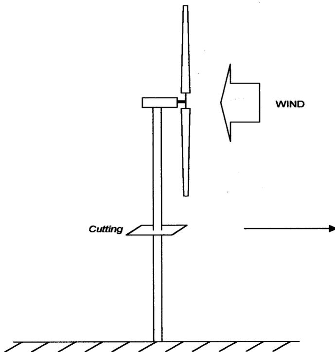
Figure 4.1: a wind turbine subjected to wind loading
