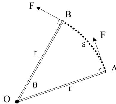
Figure 3.7: Work done by a constant torque
