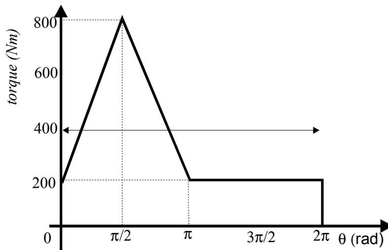
Figure 3.9: Torque requirement for Worked Example 3.12
