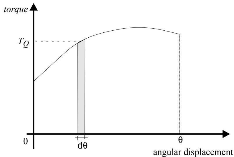
Figure 3.8: Work done by a variable torque
