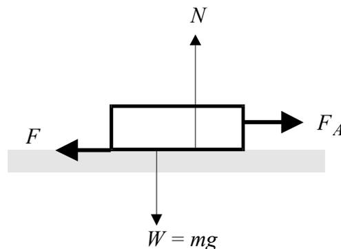
Figure 2.4: A block on a rough surface with frictional resistance to sliding
