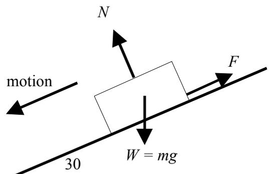
Figure 2.5: A crate sliding down a slope. Worked Example 2.5
