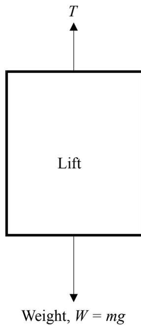
Figure 2.1 Lift and force direction for Worked Example 2.4
