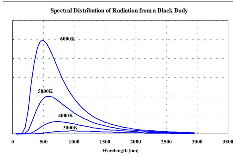
**Figure 3:** The spectral distribution of emission from a black body for a range of temperatures
