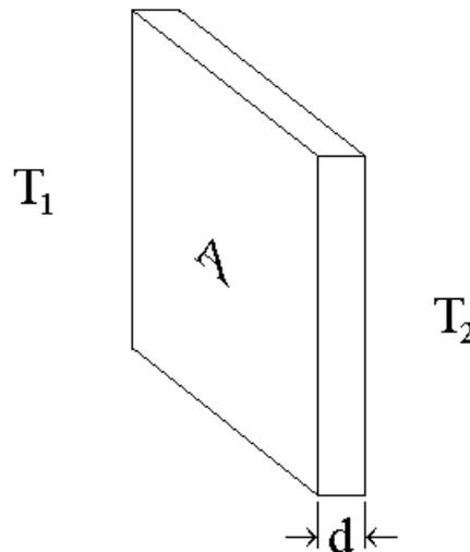
**Figure 2:** Schematic illustration of conductive heat transfer
