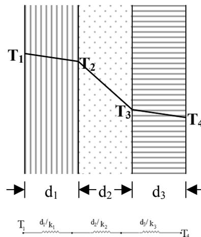
**Figure 4:** Equivalent thermal network for a composite wall
