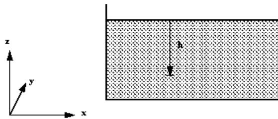
*Fluid head measurement in a tank.*
