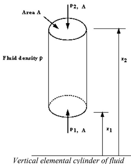
In the above figure we can see an element of fluid which is a vertical column of constant cross sectional area,  $A$ , surrounded by the same fluid of mass density  $\rho$ . The pressure at the bottom of the cylinder is  $p_1$  at level  $z_1$ , and at the top is  $p_2$  at level  $z_2$ . The fluid is at rest and in equilibrium so all the forces in the vertical direction sum to zero. i.e. we have
