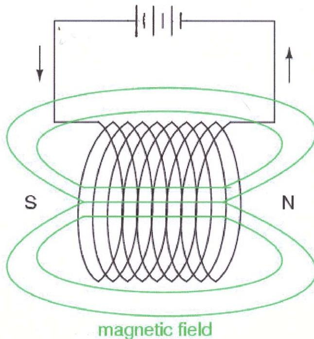
The amount of magnetic field force generated by a coiled wire is proportional to the current through the wire multiplied by the number of "turns" or "wraps" of wire in the coil. This field force is called *magnetomotive force* (mmf), and is very much analogous to electromotive force (E) in an electric circuit.
