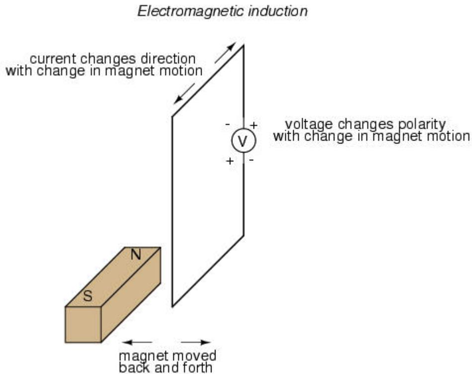
Faraday was able to mathematically relate the rate of change of the magnetic field flux with induced voltage (note the use of a lower-case letter "e" for voltage. This refers to *instantaneous* voltage, or voltage at a specific point in time, rather than a steady, stable voltage.):
