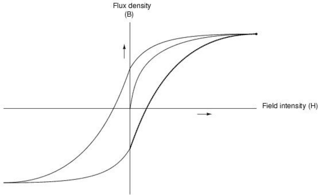
The "S"-shaped curve traced by these steps form what is called the *hysteresis curve* of a ferromagnetic material for a given set of field intensity extremes (-H and +H).
